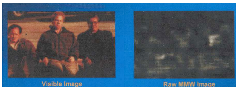
Figure 14. Visible and MMW images of a group of persons, one of whom is concealing a simulated handgun [27]
